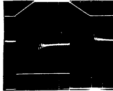
TOP TRACE OUTPUT 5V/DIV & 2.0 \mu SEC/DIV CENTER TRACE DIFFERENTIAL COMPARISON OF INPUT AND OUTPUT 2mV/DIV - 0 VOLTS THROUGH CENTER - 2.0 \mu SEC/DIV BOTTOM TRACE INPUT 5V/DIV & 2.0 \mu SEC/DIV
