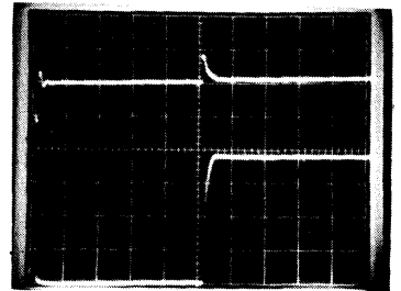
(b) TRANSIENT RESPONSE TOP TRACE: OUTPUT VOLTAGE (200 mV/DIV AND 5 μs/DIV) BOTTOM TRACE: COLLECTOR OF LOAD SWITCHING TRANSISTOR, LOAD = 1 AMPERE (5 VOLTS/DIV AND 5 μs/DIV)
