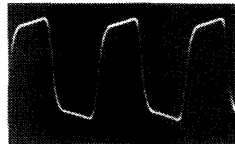
Fig. 17(c) - CA3070 terminal No. 8, oscillator waveform 1.6 V p-p 3.58 MHz.
