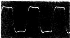
Fig. 17(b) - CA3070 terminal No. 7, oscillator waveform 1.4 V p-p 3.58 MHz.
